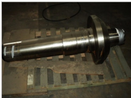
Emsco LB 650 Swivel Stem extended length
